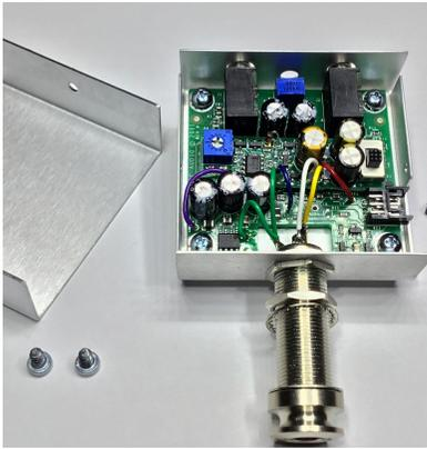
The **Amulet M Plus™** has new features and to access these new features, remove the two screws on the sides of the preamp and remove the lid. Here you will find the new **Gain Trimmer** and **Phase Switch**.
