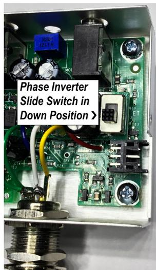
The **Phase Switch** is an internal slide switch that allows you to invert the phase of your signal, so you can perfectly match any additional pickups you might use with your instrument in a multi-system setup. This can also be used to help to increase gain before feedback in difficult monitoring situations.
