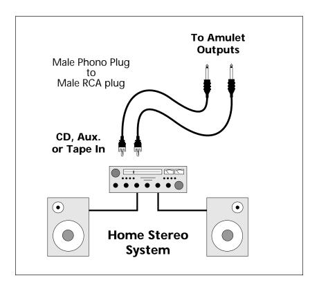
You can also use a home stereo setup for a sound system, provided that the speakers are designed for heavy duty use. Guitar playing can be hard on ordinary stereo speakers (especially using the Amulet system, since it is designed to deliver every bit of energy to the amplifier). If your stereo speakers flap wildly and make horrible grinding noises whenever you strum hard...TURN IT DOWN.
