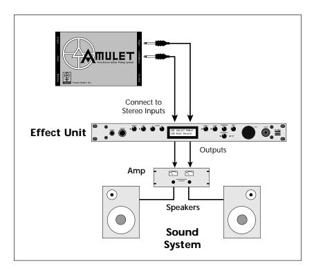
If you don't have a mixer, you can plug the Amulet outputs directly to a stereo effect unit and then to the power amp. A stereo equalizer can also be used if desired.
