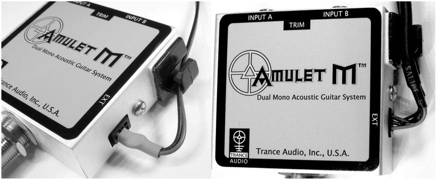
**The clip on the side of the Amulet M preamp** (adjacent to the EXT jack where the cable/battery clip plugs in) allows you to securely anchor the cable to the preamp and prevent it from being pulled loose or disconnected by vibration or cable routing problems.
